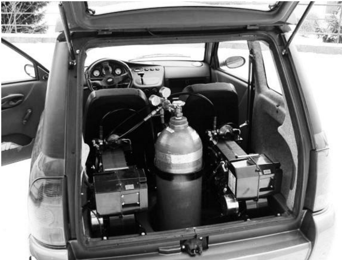
Fig. 2: Hydrogen fuel cells Nexa build in a hydrogen car SEM H2.
