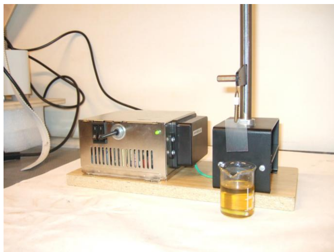
Fig. 1: Dip-coating laboratory apparatus.
