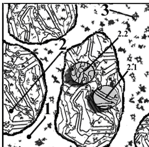
Fig. 4 Conceptual supramolecular structure of C-PEM based on S-PA and ZrP, where: 1 - amorphous parts of the polymer matrix; 2 - «quasi-crystalline» domains; 3 - nanoparticles of ZrP.
