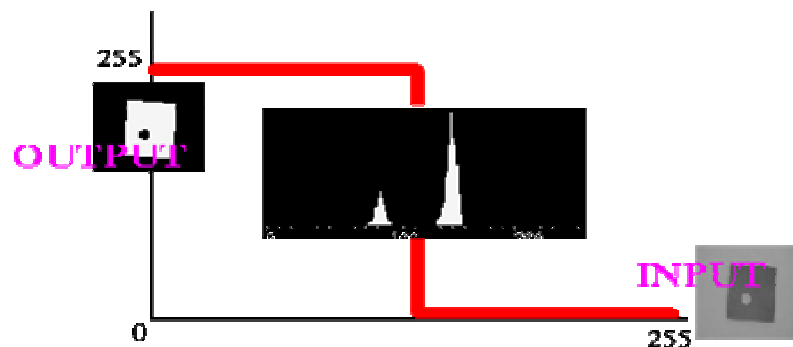
Fig. 1 Usage of thresholding for image preparation for analyzing.
