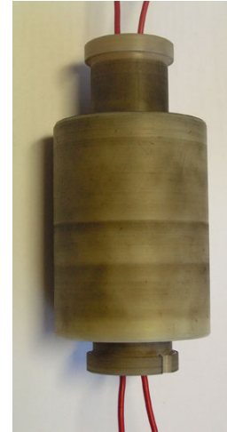
Fig. 1 a) Measuring piston (front view) with a measured sample b) Measuring piston without sample c) Real piston
