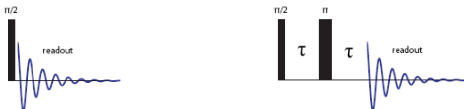
Fig. 5 Signal sequence for direct FID signal Fig. 6 Signal sequence for Hahn echo signal after HF pulse
