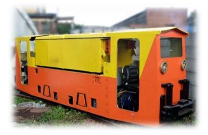
Figure 2. ELA-44 mine battery locomotive
