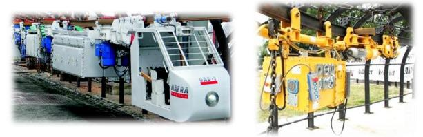
*Figure 3.* (*left*) GAD-1 battery drivetrain of suspended monorail *Figure 4.* (*right*) PCA-1 suspended battery drivetrain
