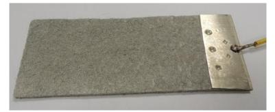
*Figure 4.* Monometallic tin felt electrode ready for filling (non-woven PP textile carrier realized by needling).
