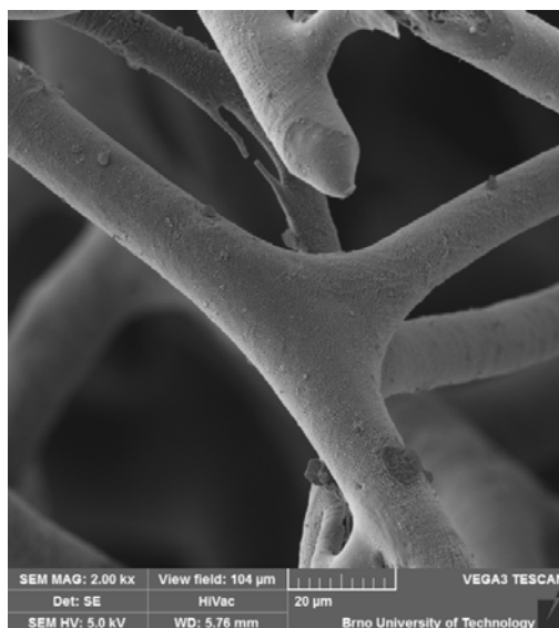
Figure 1. SEM analysis of the Spongia officinalis after annealing, view field 104 \mu\text{m} .
