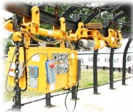
**Figure 3.** (left) GAD-1 battery drivetrain of suspended monorail
