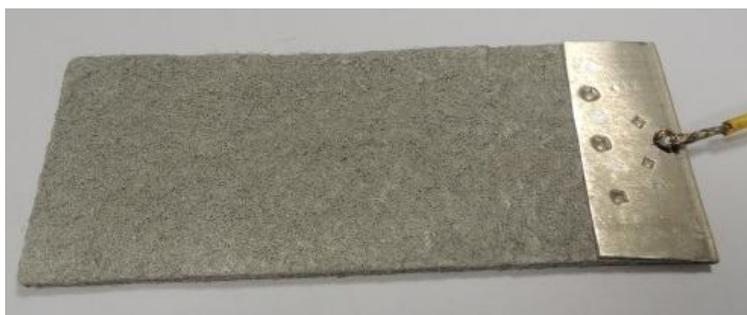
**Figure 4.** Monometallic tin felt electrode ready for filling (non-woven PP textile carrier realized by needling).
