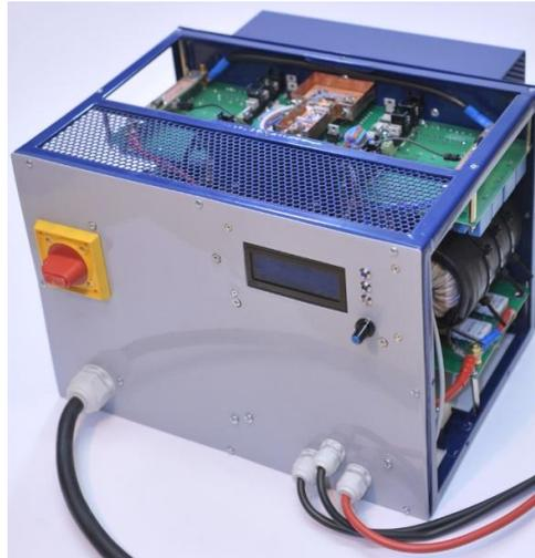
**Figure 1.** Total view of the charger device (without upper cover)
