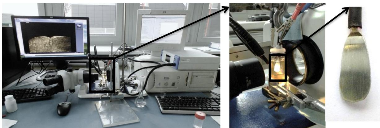
**Figure 1.** System for measuring Zn dendrite growth
