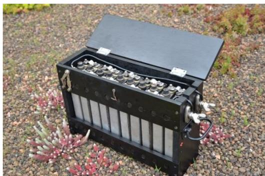
**Figure 5.** View of the renovated accumulator
