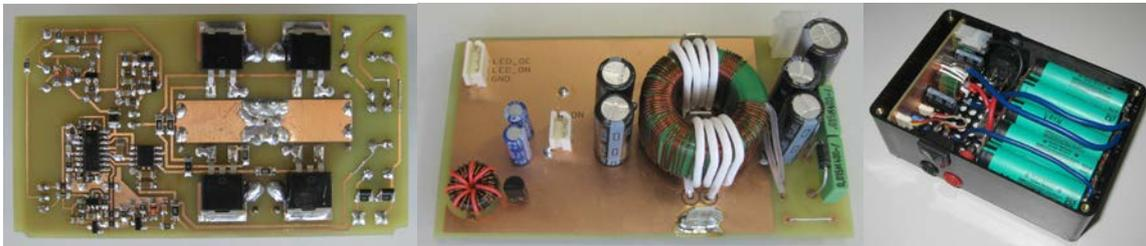
**Figure 3.** Voltage converter board (left and middle) and a finished prototype (right).
