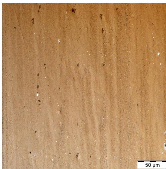
**Figure 2.** Microstructure of sample core B, etched hydrofluoric acid 0,5%
