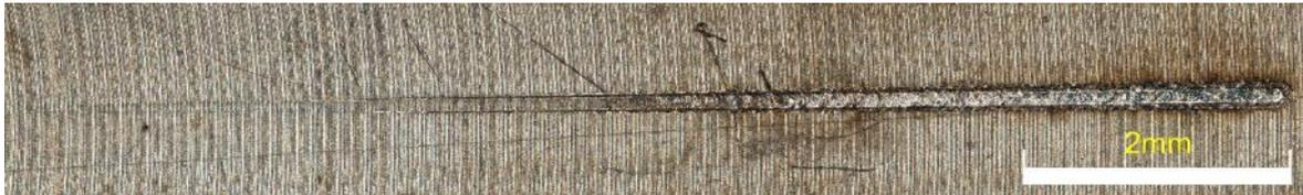
**Figure 6a.** The record of the scratch test sample B-DLC
