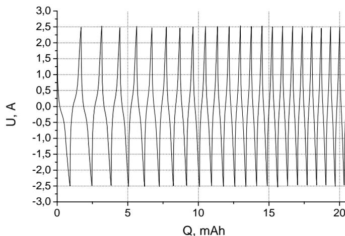
**Fig.2** The cycling history of SWNT-supercapacitor with current density 0.5 A.g<sup>-1</sup>.
