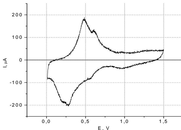
**Fig.3** CVA for electrode from ST10 (scan rate  $0.075 \text{ mV.s}^{-1}$ , weight of ST10 0.6 mg)
