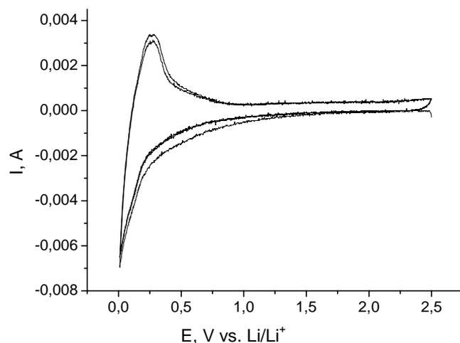
**Fig.1** CVA for electrode from SWNT (scan rate 1 mV.s<sup>-1</sup>)
